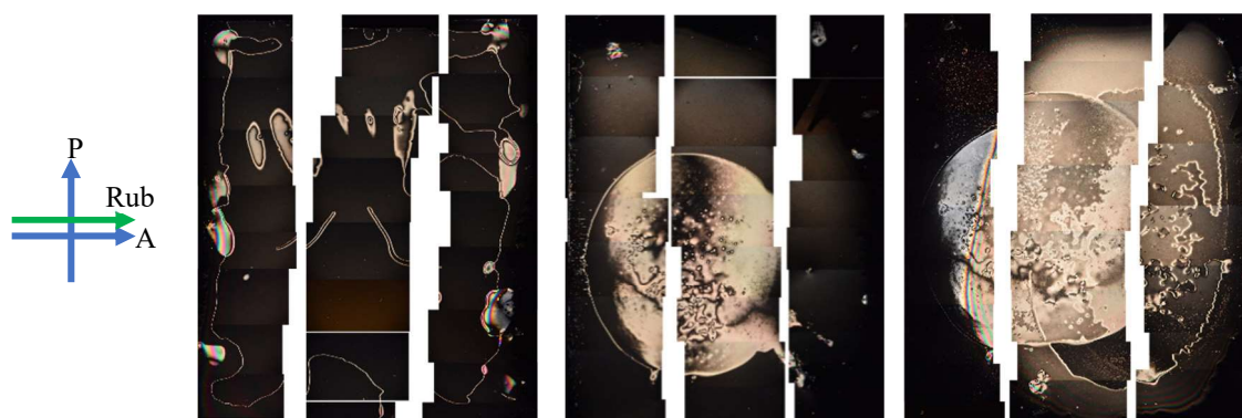
Figure 1- Demonstrative composite transmission polarized optical microscopy images of 8.8 \pm 0.1 \mu\text{L} NLC confined in a 20 \times 16 \text{mm} rectangle with (left) no RM82/MBF, (middle) UV cured RM82/MBF, and (right) middle system annealed. The rubbing direction is approximately aligned with one of the crossed polarisers.
