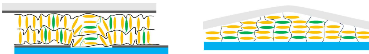
Figure 1. a) Liquid crystal elastomer lens made using a hole patterned electrode between ITO coated PET film and glass. The liquid crystal is represented by the yellow molecules and the green represents the crosslinker. A strong voltage is applied to the system aligning the liquid crystal elastomer so that a gradient can be made in the refractive index, creating a lensing effect. This can then be cured using UV light to maintain the alignment. b) Liquid crystal elastomer lens made using a lens shaped mould. The liquid crystal is represented by the yellow molecules and the green represents the crosslinker. Due to the liquid crystal's birefringence the lens will have two different focal points depending on the polarisation orientation of the input light.
