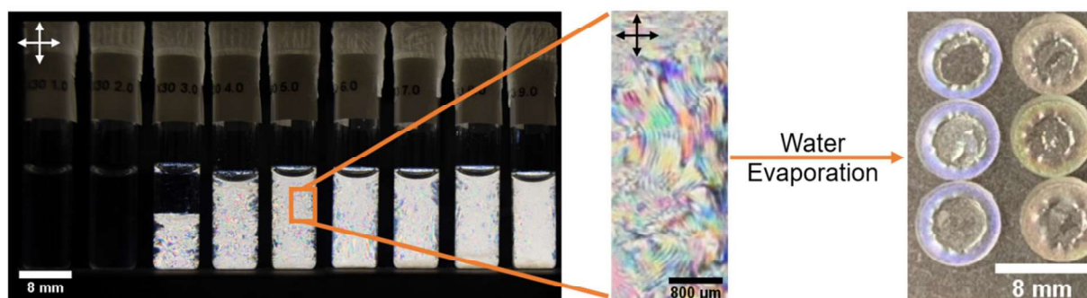
Figure 1: From left to right: Aqueous mixtures with 1 to 9 wt% of treated xanthan between crossed polarizers. Fingerprint texture of a sample with 5 wt% of treated xanthan between crossed polarizers. Dried xanthan films exhibiting selective reflection.
