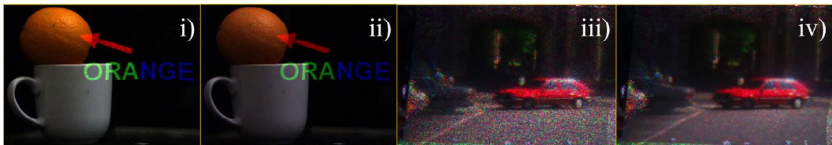
Figure 1: (Left) RGB Laser head-up display demonstrator with i) no speckle reduction, ii) active speckle reduction from a transmissive configuration LC device. (Right) RGB Laser projector demonstrator with i) no speckle reduction, ii) active speckle reduction from a reflective configuration LC device.
